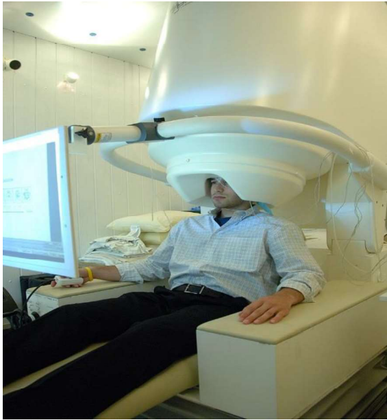
Figure 1. 5- Magnetoencephalogram recording machine. An array SQUID is located in the helmet like structure supercooled with liquid helium. In front of the participant is the screen for stimulus display
